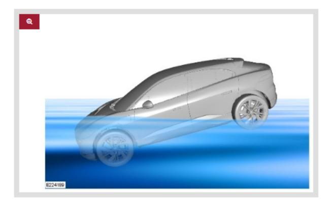
Persons handling the recovery of a BEV must wear appropriate PPE, as detailed by your local authority, until the High Voltage (HV) system has been correctly powered down.
