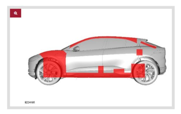
The sills must be supported during cutting and extrication procedures. If a ram must be deployed, place blocks under the sill around the area where force is applied. If a suitable jacking point cannot be located, support the sills and deflate the tires.
